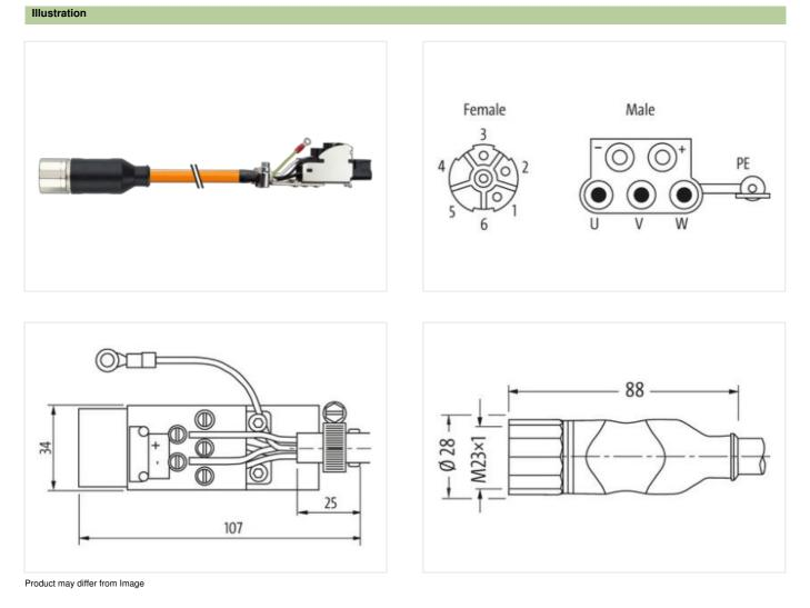
Cable length 21 m Side 1 Tightening torque 2 Nm Family construction form M23 Thread M23 x 1 Width across flats SW27
